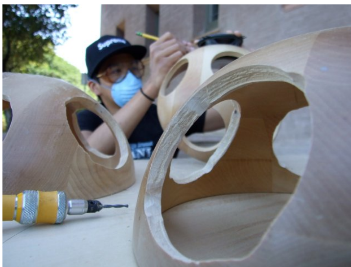
Figure 2.11: Making speakers from salad bowls. The holes are for mounting car speaker drivers. [115]
