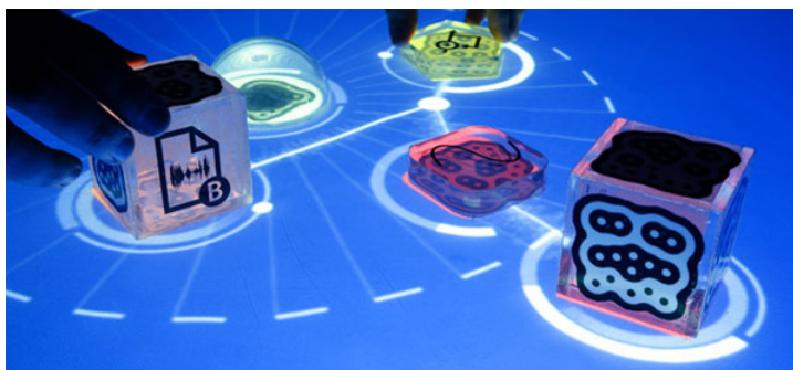
Figure 2.5: The reacTable modular synthesizer is controlled with blocks and multi-touch.
