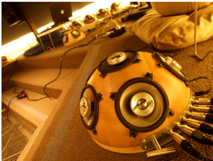
Figure 2.12: A finished SLOrk speaker with six car speaker drivers, audio cable connections, power connection, and carrying handle. [115]
