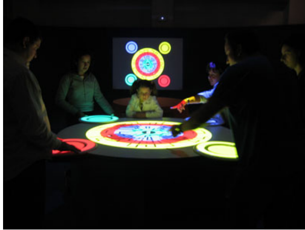
Figure 3.4: The Jam-o-Drum in use [3]. Note how the interface is projected onto the outstretched arm of one of the players.
