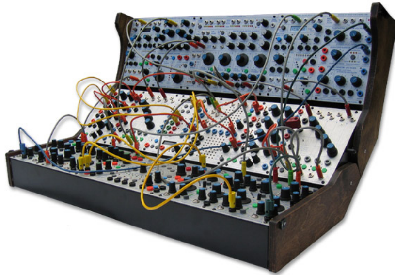
Figure 2.3: A Buchla analog synthesizer with knobs, buttons, and cables for changing the basic sound of the synthesizer.
